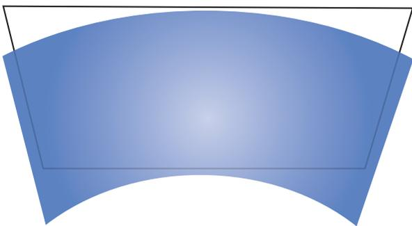
The reason why this is done is related to the fact that the **theoretical screen gain only applies when looking perpendicular at the screen**. The theory of half-gain angle explained how the perceived luminance drops as you see the screen under larger angles. These viewing angles increase as you sit further to the edges of the auditorium, or as you look
